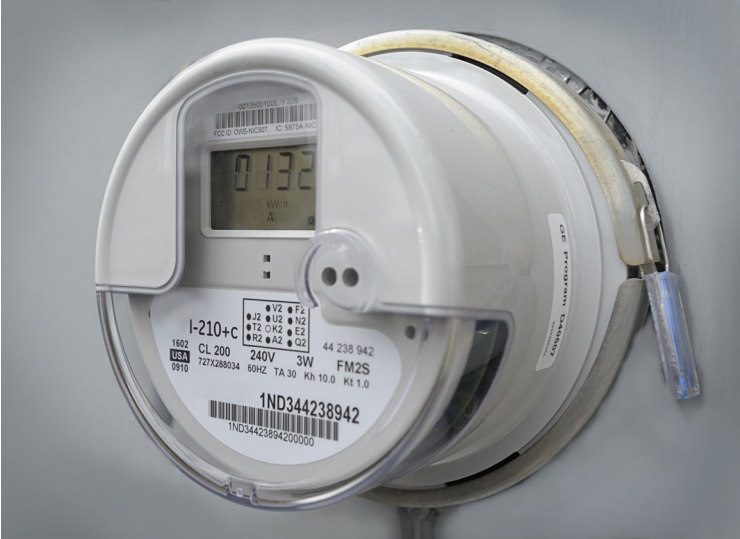
Photo of a smart meter, a central component of AMI technology which enables electric customers to better manage their energy usage, among other benefits.
